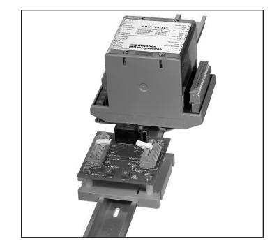
power supply that can provide 24VDC excitation power at 150mA to drive input sensors. The SPC-701 and SPC-704 have a signal averaging potentiometer that helps alleviate false trips during sudden signal changes. These controllers have easy to view bright LEDs that show the relay and Power On status. The relay outputs can handle up to 3A.
