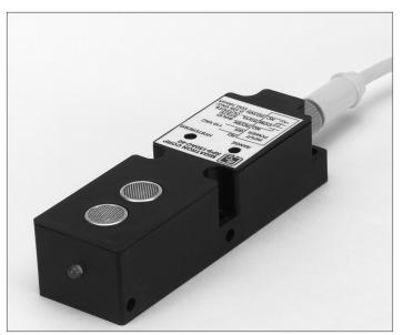
disconnect (QD) cable receptacle. The housing is constructed of PBT plastic and has standard 30mm x 60mm limit switch mounting dimensions, as well as side holes for mounting the sensor on its side. The output consists of two solid state relays N.O. and N.C., that can switch 2 - 130VAC or VDC up to 50mAAC or 100mADC continuous. The relay outputs are short circuit protected and isolated up to 1500VRMS.
