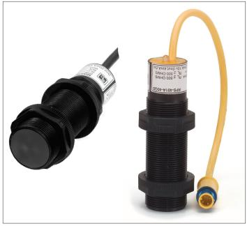
the target. Yellow indicates a weak signal and bright red indicates a strong signal. The transducer frequency for the RPS-401A is 175kHz for the 4 - 40" range and 150kHz for the 8 - 80" range. The RPS-401A housing is constructed of PVC plastic. See the RPS-426A data sheet for the Stainless Steel version. The housing measures 30 mm x 104 mm. A standard 6' cable is provided, or a quick disconnect (QD) version is also available.
