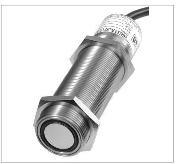
the target. Yellow indicates a weak signal and bright red indicates a strong signal. The transducer frequency for the RPS-426A is 175kHz for the 4 - 40" range and 150kHz for the 8 - 80" range. The RPS-426A housing is constructed of Stainless Steel. See the RPS-401A data sheet for the PVC plastic version. The housing measures 30 mm x 104 mm. A standard 6' cable is provided, or a quick disconnect (QD) version is also available.
